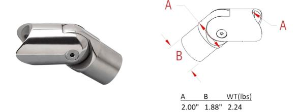
This adjustable elbow is made of 316 grade stainless steel, has a satin (brushedfinish, and is designed to mount on the *outside* of a 2" OD tube on one side of the fitting. The other side of the fitting is designed to fit *inside* a 2" OD tube with a 0.06" thick wall. Mount the first side with a fastener or by welding. Connect the second side with adhesive.
