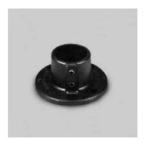
Item 55BK-28090 is made of aluminum-magnesium alloy 535, has a matte black powder coat finish, and includes two screws to hold the pipe in place. It is designed to hold 1-1/2" IPS pipe (see item A112ID).
