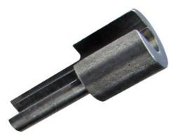
The PL-Key is primarily used when you want to remove the cable from the Push-/Pull-Lock during the installation and cable-trimming process. Because it opens the spring-loaded jaws, it also helps you insert the cable into the Push-/Pull-Lock if you're having trouble.
