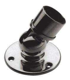
This adjustable angle flush flange is available in brass and two different grades of stainless steel. It is a two part fitting with the two parts held together by a screw at the pivot point.
