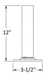
The 20-541/1H flange and insert set is made of cast iron and steel and is designed to mate with 1-½" round tube (item A110). The flange has four holes for mounting hardware and a large threaded hole in the middle that mates with the threaded end of the insert.
