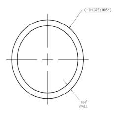
The 20-A110SL steel insert has a 1-3/8" outside diameter and fits inside 1-1/2" x 0.05" wall architectural tube. The insert serves to reinforce the tube and is available in 12 foot stock lengths.
