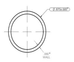
The 20-A100SL steel insert has a 7/8" outside diameter and fits inside 1" x 0.05" wall architectural tube. The insert serves to reinforce the tube and is available in 12 foot stock lengths.
