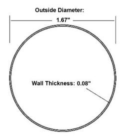
47-A114 architectural round tube is a stainless steel tube with a 1.67" outside diameter, a 0.08" wall thickness, and is available in stock lengths up to 20 feet. It is made with 316 grade stainless steel.
