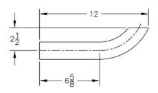
49301R Wall Return Bend RIGHT is made of aluminum, is designed to connect to 1-1/2" IPS schedule 40 pipe, and has an anodized finish.
