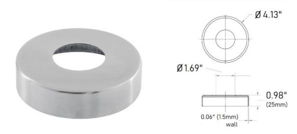
The 49-540/424 round flange canopy or escutcheon plate is made of 316 grade stainless steel, has a satin (brushed) finish and allows for a 1.67" diameter round tube to pass through its center hole. Use this cover as a decorative addition to flanges that are often unseemly because of the mounting hardware used with them.
