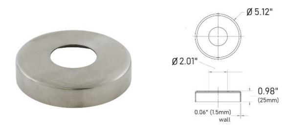
The 49-540/2 round flange canopy or escutcheon plate is made of 316 grade stainless steel, has a polished finish and allows for a 2" diameter round tube to pass through its center hole. Use this cover as a decorative addition to flanges that are often unseemly because of the mounting hardware used with them.
