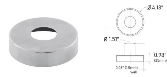
The 49-540/1H round flange canopy or escutcheon plate is made of 316 grade stainless steel, has a satin (brushed) finish and allows for a 1-1/2" diameter round tube to pass through its center hole. Use this cover as a decorative addition to flanges that are often unseemly because of the mounting hardware used with them.
