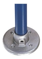
A heavy duty flange, with wide base, for spreading loads over a large surface area. This flange, with holes provided for countersunk flat head screw fixings only, is for use on structures where the fixing required is positional only. Frequently used as a wall fixing bracket. Ø indicates diameter of fixing holes. It is not recommended for use as a base flange to support guardrailing or balustrading.
