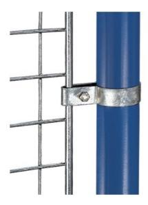
Single clips for attaching wire-mesh infilling. For economy it is possible to use Type 81 clips without the safety attachment, to secure various types of infill panels (plyboard, perspex, etc.) up to a thickness of 25/64". All clips are supplied with hexagonal head fixing bolts, M6x35mm long, and nut.
