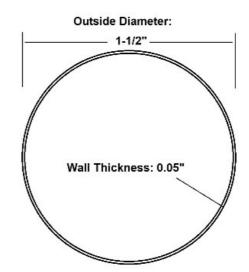
40-A110 architectural round tube is a stainless steel tube with a 1-1/2" outside diameter, a 0.05" wall thickness, and is available in stock lengths up to 20 feet. It is made with 304 grade stainless steel.
