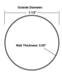
40-A110 architectural round tube is a stainless steel tube with a 1-1/2" outside diameter, a 0.05" wall thickness, and is available in stock lengths up to 20 feet. It is made with 304 grade stainless steel.
