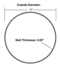
44-A100 architectural round tube is a stainless steel tube with a 1" outside diameter, a 0.05" wall thickness, and is available in stock lengths up to 20 feet. It is made with 304 grade stainless steel and has a linear brush direction with a #4 grit.
