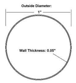
00-A100 architectural round tube is a brass tube with a 1" outside diameter, a 0.05" wall thickness, and is available in stock lengths up to12 feet. It is made with C2680 alloy brass and conforms with ASTM B36.
