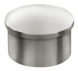
The 40-600/1H flush end cap is made of 304 grade stainless steel, has a polished finish and provides a simple and smooth, flush finish to the end of a tube.
