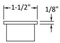
The 00-600/1H flush end cap is made of brass, has a polished finish and provides a simple and smooth, flush finish to the end of a tube.
