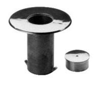
The 545 floor socket with cap is the fitting to use for removable railing and queueing posts. It is designed to hold 2" round tube and has a receiving space that is just over 2" in inside diameter to receive the tube. It is available in brass and 304 grade stainless steel and it mounted into the ground - typically core drilled into concrete. This item includes a cap to close the opening when there is no post in place.
