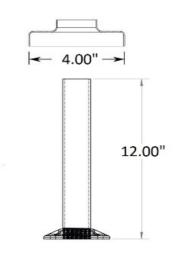
44-B/1H flange, insert, and canopy set is made of a cast iron flange, a steel insert, and a satin (brushed) stainless steel canopy. This set is designed to mate with 1-1/2" OD round tube. The flange has four holes for mounting hardware and a large threaded hole in the middle that mates with the threaded end of the insert.
