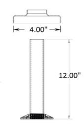
00-B/1H flange, insert, and canopy set is made of a cast iron flange, a steel insert, and a polished brass canopy. This set is designed to mate with 1-1/2" OD round tube. The flange has four holes for mounting hardware and a large threaded hole in the middle that mates with the threaded end of the insert.
