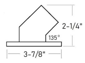
This 45 degree angle flange is an optimal solution to build angled sneeze guards or to terminate a tube from a 45 degree angle to a wall. 00-515/1H is made of polished brass and is for tube size 1-1/2" OD x 0.05" wall. The mounting flange has three counter sunk holes.
