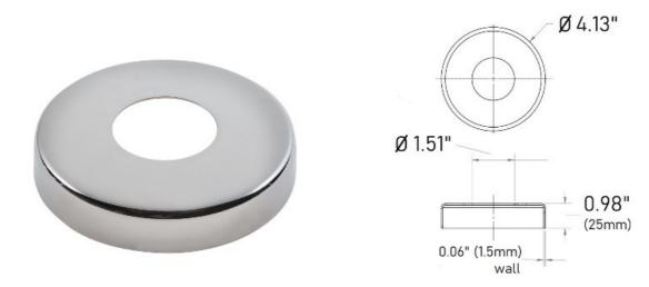
The 40-540/1H round flange canopy or escutcheon plate is made of 304 grade stainless steel, has a polished finish and allows for a 1-1/2" diameter round tube to pass through its center hole. Use this cover as a decorative addition to flanges that are often unseemly because of the mounting hardware used with them.
