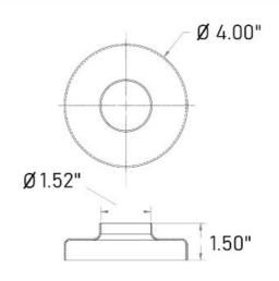
The 00-540/1H round flange canopy or escutcheon plate is made of brass, has a polished finish and allows for a 1-1/2" diameter round tube to pass through its center hole. Use this cover as a decorative addition to flanges that are often unseemly because of the mounting hardware used with them.
