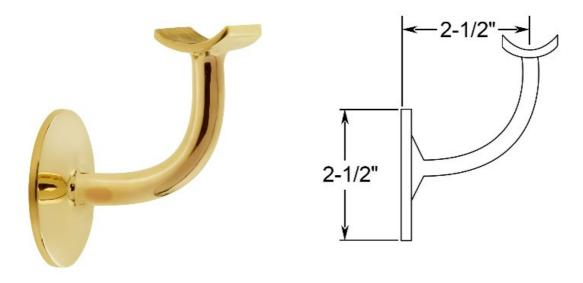
The 00-301u/1H concealed (undrilled) wall mount handrail bracket is ideal for level and stair applications. It can be mounted horizontally at a landing or at the end of a ramp. It can also be mounted at an angle for stair or ramp applications. This bracket is made of brass and has a polished finish.
