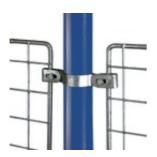
Double clips for attaching wire-mesh infilling. For economy it is possible to use Type 82 clips without the safety attachment, to secure various types of infill panels (plyboard, perspex, etc.) up to a thickness of 25/64". All clips are supplied with hexagonal head fixing bolts, M6x35mm long, and nut. Ø indicates diameter of the safety attachment bolt hole. The primary clip has a slot measuring 8mm x 15mm.
