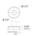
The 47-540/1H round flange canopy or escutcheon plate is made of 316 grade stainless steel, has a polished finish and allows for a 1-1/2" diameter round tube to pass through its center hole. Use this cover as a decorative addition to flanges that are often unseemly because of the mounting hardware used with them.
