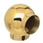
Ball fittings are used to construct handrails, footrails, stair rails, bar rails, ballet rails, and many other metal railing systems. The vertical posts of the railings should be made with a continuous architectural metal tube (for strength) while the horizontals are cut and fit with architectural hardware between posts. Ball fittings may be available in a variety of finishes not usually found in traditional brass fittings, including white, stainless steel, and more.
