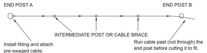
If you are bending cable across a landing, you will want to insert a Post-Protector Tube (order CS-TUBE-6 separately from Accessories) into the wood post where the cable angles out of the post. Drill a 1/4" hole 1-1/2" deep straight into the post to receive the CS-Tube.
