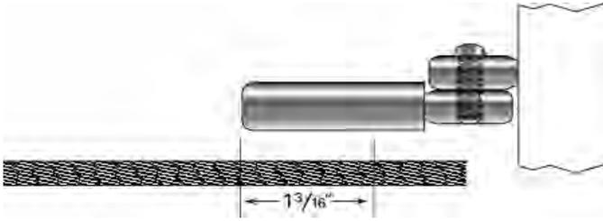
**8.** Push the cable into the hole in the fitting as far as it will go (approximately 1-1/16"). Twist the cable in a right hand direction as you push it into the fitting.
