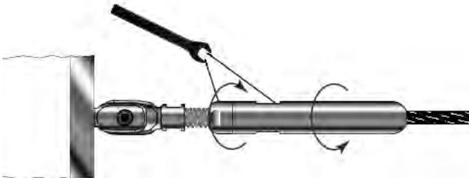
**11.** Tension in sequence, beginning with the outside cables and moving back and forth toward the center. Finished cables should be tensioned to have only 1/4" of play when finger-pulled.
