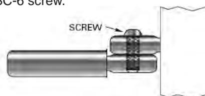
**7.** Pull the cable tightly along the side of the fitting and mark the cable 1-3/16" from the end of the fitting opposite the post. Mark and cut the cable on your mark.
