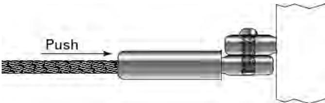
**9.** Go to the other end and tension the cable by holding it to prevent the cable from turning while you turn the Adjust-A-Body with a 7/16" open-end wrench. Be careful to protect the cable from damage while tensioning the Adjust-A-Body.
