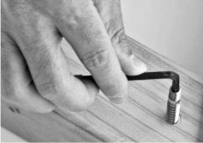
7. Thread the Push-Lock coupler onto the lag and tighten with 7/16" wrench.
