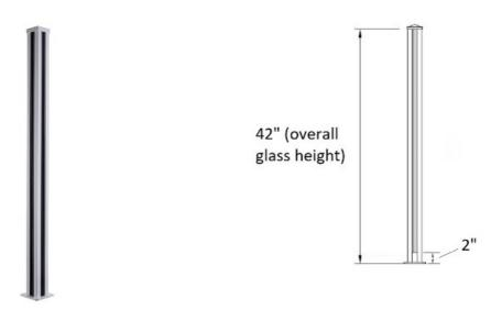
Scenic posts are made of aluminum and are 2-1/2" square in size. These posts are 42" high and have an integral channel designed to hold glass.
