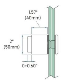
This 2"(50mm) round wall mount glass clamp from IAM Design is made of 316 grade stainless steel, has a brushed (satin) finish and is designed to hold 31/32 – 27/32" thick glass. It has an offset from the wall to the glass of 1.57" (40mm) which can be extended an additional 0.60" (15mm). Mount this bracket on a wall (recommended on a stud) using hardware appropriate for the material that it mounts on.
