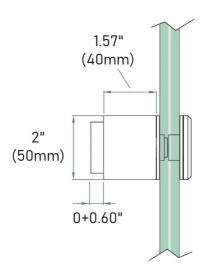
This 2"(50mm) round wall mount glass clamp from IAM Design is made of 304 grade stainless steel, has a brushed (satin) finish and is designed to hold 21/32 – 27/32" thick glass. It has an offset from the wall to the glass of 1.57" (40mm) which can be extended an additional 0.60" (15mm). Mount this bracket on a wall (recommended on a stud) using hardware appropriate for the material that it mounts on.
