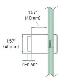
This 1.57" (40mm) round wall mount glass clamp from IAM Design is made of 304 grade stainless steel, has a brushed (satin) finish and is designed to hold 1/2 - 19/32" thick glass. It has an offset from the wall to the glass of 1.57" (40mm) which can be extended an additional 0.60" (15mm). Mount this bracket on a wall (recommended on a stud) using hardware appropriate for the material that it mounts on.
