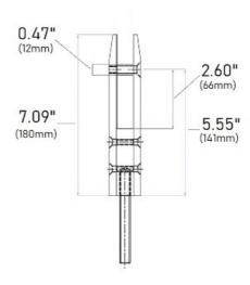
This core drill rectangular glass clamp from IAM Design is made of 316 grade stainless steel, has a brushed (satin) finish, and is designed to hold 1/2 and 11/16" thick glass. Mount in the floor with a M12 threaded bolt.
