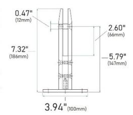
This floor mount rectangular glass clamp from IAM Design is made of 304 grade stainless steel, has a brushed (satin) finish, and is designed to hold 1/2 and 11/16" thick glass. The square flange on the bottom is 3.94" wide and has four mounting holes.
