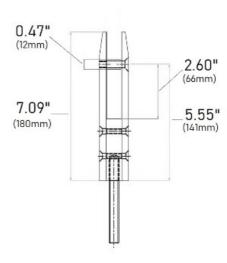
This core drill rectangular glass clamp from IAM Design is made of 304 grade stainless steel, has a brushed (satin) finish, and is designed to hold 1/2 and 11/16" thick glass. Mount in the floor with a M12 threaded bolt.
