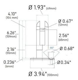
This floor mount round glass clamp from IAM Design is made of 304 grade stainless steel, has a brushed (satin) finish, is 1.93" (49mm) in diameter, and is designed to hold 1/2 and 11/16" thick glass. The flange on the bottom is 3.94" in diameter and has three countersunk holes for mounting to the floor.
