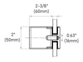
This 2"round wall mount glass clamp from IAM Design is made of 316 grade stainless steel, has a brushed (satin) finish and is designed to hold 5/16 - 21/32" thick glass. It has an offset from the wall to the glass of 2-3/8" (60mm). Mount this bracket on a wall (recommended on a stud) or on a rectangular vertical post using hardware appropriate for the material that it mounts on.
