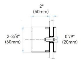
This 2-3/8" round wall mount glass clamp from IAM Design is made of 316 grade stainless steel, has a brushed (satin) finish and is designed to hold 5/16 - 21/32" thick glass. It has an offset from the wall to the glass of 2" (50mm). Mount this bracket on a wall (recommended on a stud) or on a rectangular vertical post using hardware appropriate for the material that it mounts on.
