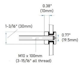
This 1-3/16" round wall mount glass clamp from IAM Design is made of 316 grade stainless steel, has a brushed (satin) finish and is designed to hold 5/16 - 21/32" thick glass. It has an offset from the wall to the glass of 0.38" (10mm) and comes complete with a threaded bolt. Mount this bracket on a wall (recommended on a stud) or on a rectangular vertical post using the included hardware or alternate depending on the material the bracket is being mounted upon.
