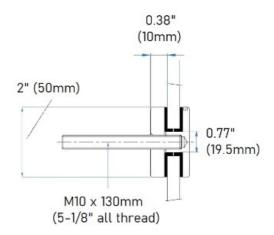
This 2"round wall mount glass clamp from IAM Design is made of 304 grade stainless steel, has a brushed (satin) finish and is designed to hold 5/16 - 21/32" thick glass. It has an offset from the wall to the glass of 0.38" (10mm) and comes complete with a threaded bolt. Mount this bracket on a wall (recommended on a stud) or on a rectangular vertical post using the included hardware or alternate depending on the material the bracket is being mounted upon.
