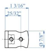
The standoff crossbar holder is made of stainless steel, has a brushed (satin) finish and is designed to hold a 12mm OD round rod or tube. Mount this standoff on a square tube.
