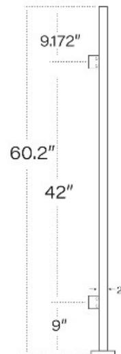
The 60" high floor mount partition post is made of 2" square tube and 316 grade satin (brushed) stainless steel. This end post comes with a flange welded at the bottom, a flange canopy, two glass grips attached to the post and a flush end cap on the top.
