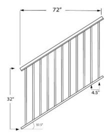
This 6ft long Stair Picket Rail Panel is designed for 36" high railing and it has 3/4" square pickets that are spaced 3-3/4" apart to pacify the 4" sphere rule. This panel has a white painted finish.
