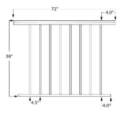
This 6ft long Level Picket Rail Panel is designed for 42" high railing and it has ¾" square pickets that are spaced 3-3/4" apart to pacify the 4" sphere rule. This panel has a dark bronze painted finish.
