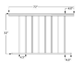
This 6ft long Level Picket Rail Panel is designed for 36" high railing and it has ¾" square pickets that are spaced 3-3/4" apart to pacify the 4" sphere rule. This panel has a black painted finish.
