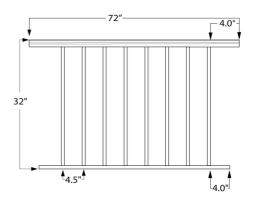
This 6ft long Level Picket Rail Panel is designed for 36" high railing and it has ¾" square pickets that are spaced 3-3/4" apart to pacify the 4" sphere rule. This panel has a white painted finish.
