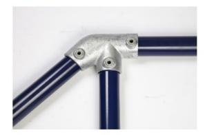
Tee Fitting designed for the top rail on guardrail on slopes and staircases between 30° and 45° at the junction where the handrail changes from level to sloping down the stairs
